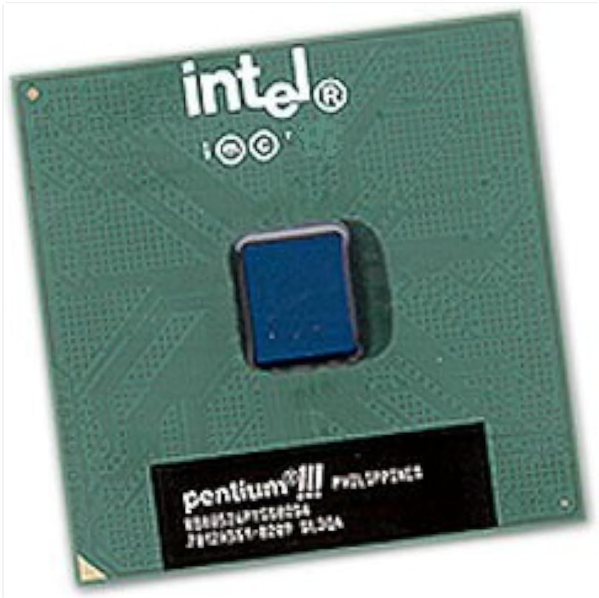
Figure 1: A top-down view of the Intel Pentium III processor. The green ceramic package features the Intel logo and 'Pentium III' branding, with the central silicon die visible as a small blue square.
