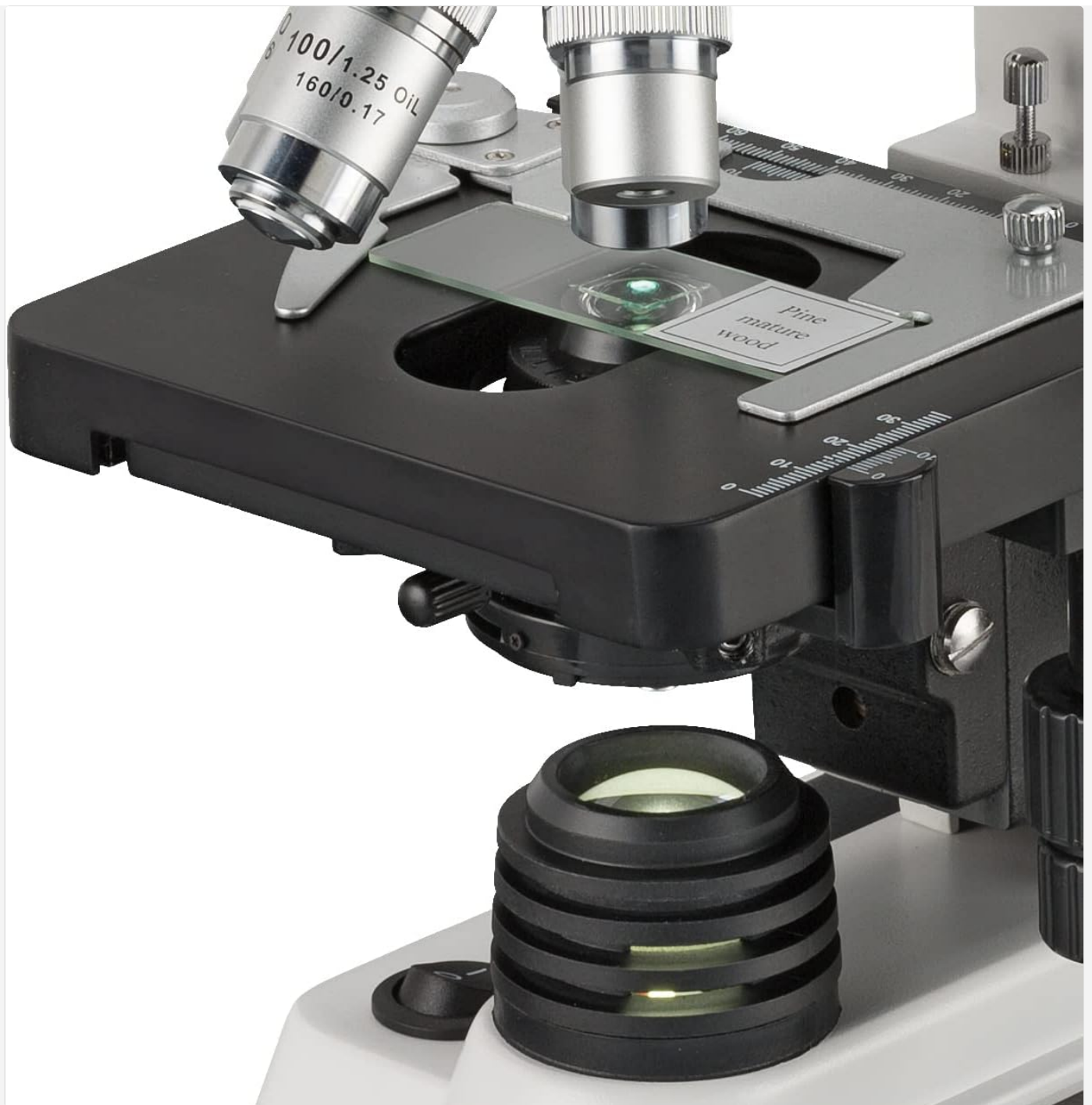
Image 5.1: Close-up view of the objective lenses mounted on the revolving nosepiece, positioned above the mechanical stage with a specimen slide.
