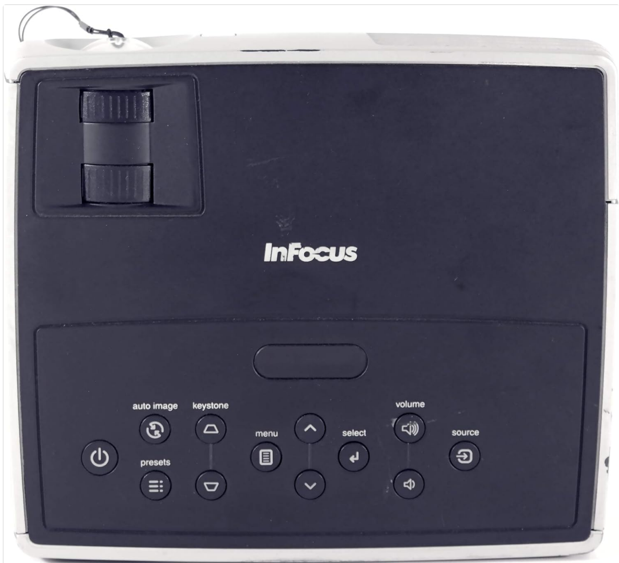
Figure 4: Top Panel and Control Keypad. This image provides a top-down view of the projector, showcasing the LiteTouch™ control panel with buttons for power, auto image, keystone, menu, select, volume, and source selection. The
