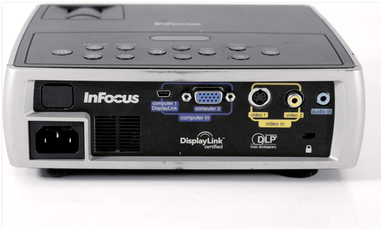
Figure 3: Rear Panel with Connectivity Ports. The rear panel of the InFocus IN1102 is shown, highlighting the various input ports including DisplayLink USB, VGA (Computer 1 and Computer 2), Video 1 (S-Video), Video 2 (Composite), and Audio In. The power input socket is on the far left.
