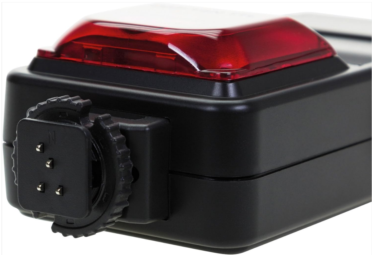
Figure 4.3: Detail of the hot shoe mount on the DAF-14 control unit, used for attaching the flash to a Nikon DSLR camera.
