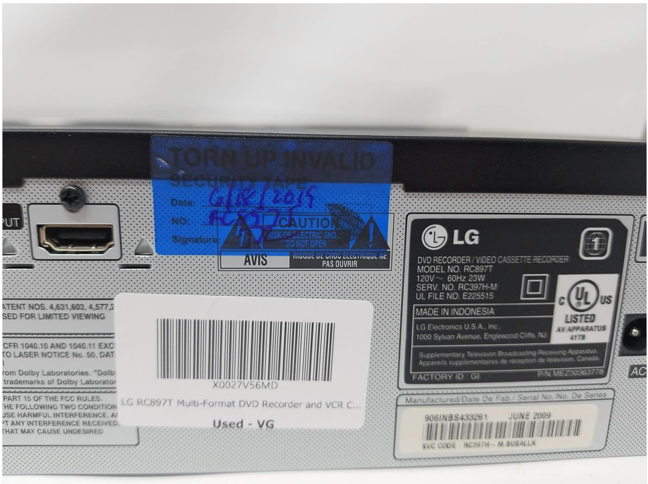
Image: The rear panel of the LG RC897T, displaying connection ports such as HDMI, component, composite, and antenna inputs. The product label with model and electrical specifications is also visible.
