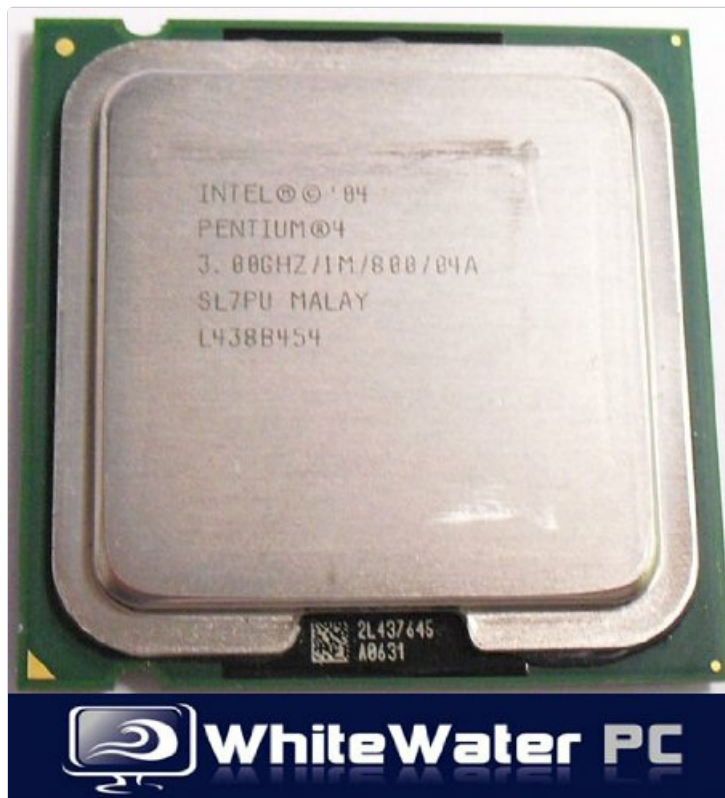
Image: Intel Pentium 4 3.0GHz 800MHz 1MB Socket 775 CPU, showing the top view of the processor with its heat
