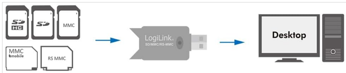
Image 3.2: A diagram illustrating the connection process: various memory card types (SD, SDHC, MMC, RS-MMC) are inserted into the Logilink card reader, which then connects to a desktop computer for data transfer.
