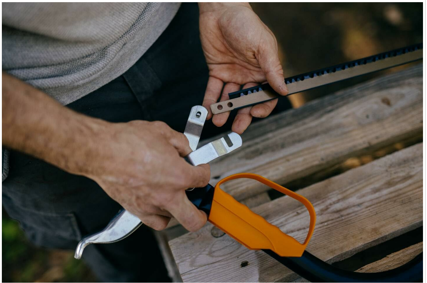
Image 4.3: Hands carefully inserting the saw blade into the tensioning mechanism at the handle end of the bow saw, showing the final step of blade attachment.
