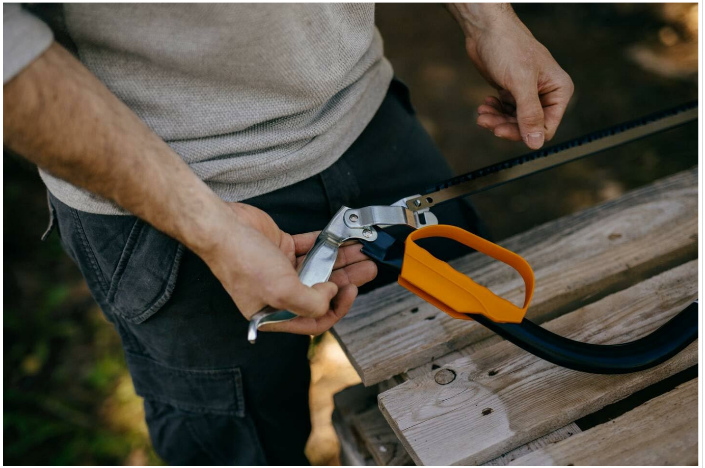
Image 4.2: A close-up of hands holding the saw handle and a new blade, demonstrating the initial step of aligning the blade for installation.
