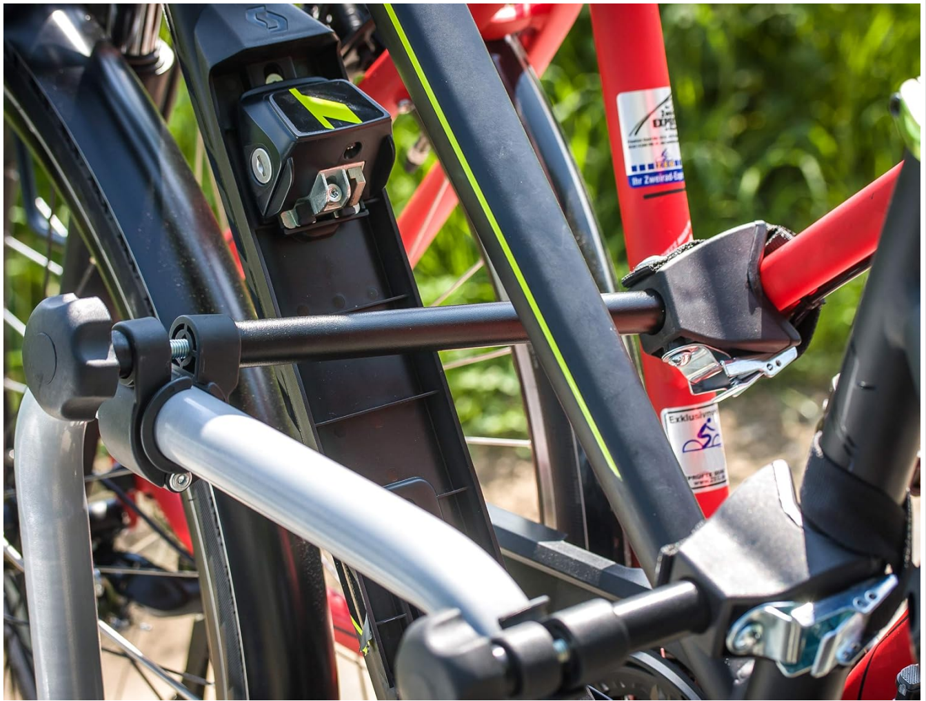
Image: A close-up view of a bicycle frame being secured by the carrier's adjustable frame holder.
