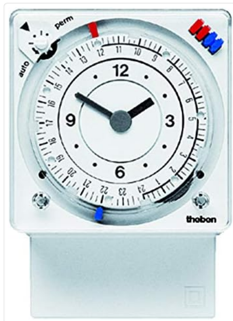
Figure 1: Theben SYN 269 h Analogue Time Switch. This image displays the front view of the Theben SYN 269 h Analogue Time Switch. It features a central clock face with hour and minute hands, surrounded by a 24-hour dial. The dial has segments for setting daily or weekly programs using small, movable pins (red and blue). On the top left, there is a selector switch labeled 'auto' and 'perm' for automatic or permanent operation. The 'thobon' (likely Theben) brand name is visible on the bottom right of the dial.
