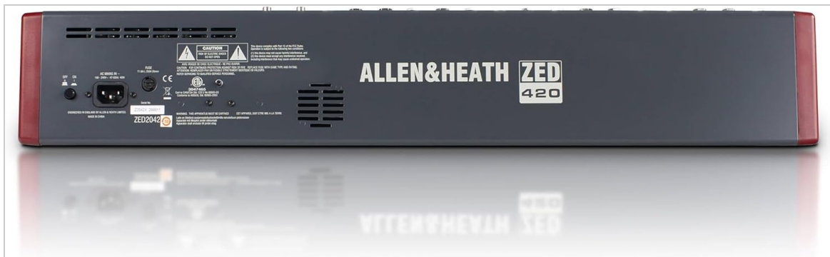
Image: Rear panel of the ZED-420 mixer, highlighting the power input and other rear connections.
