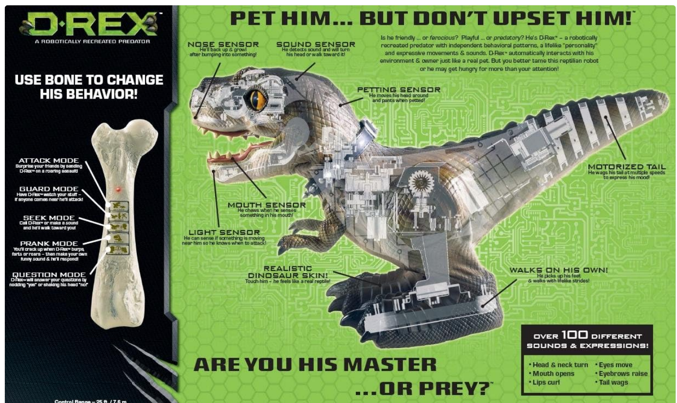
Figure 5: D-Rex internal components and sensor locations.
