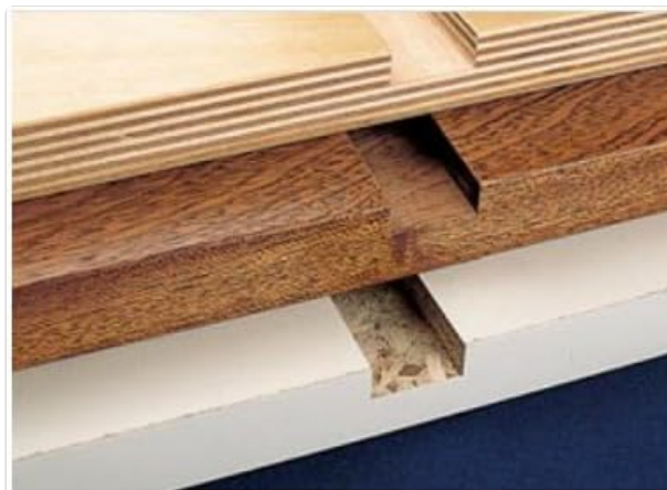
Figure 4: Examples of precise dado cuts achieved with the CMT Precision Dado Set in various wood types.
