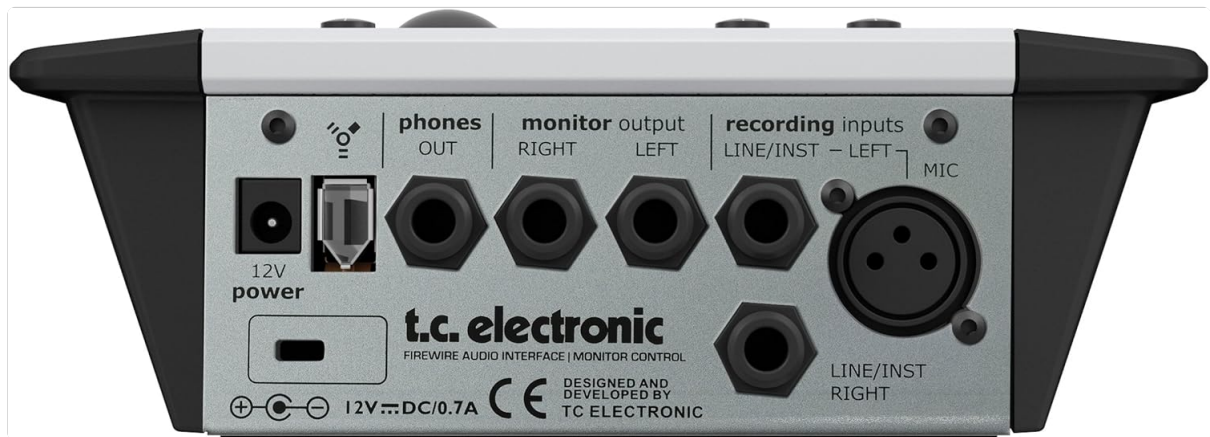
Figure 3.2.1: Rear panel connections of the Desktop Konnekt 6, illustrating power, Firewire, monitor outputs, headphone output, and various input types including XLR for microphone and 1/4" jacks for line/instrument.
