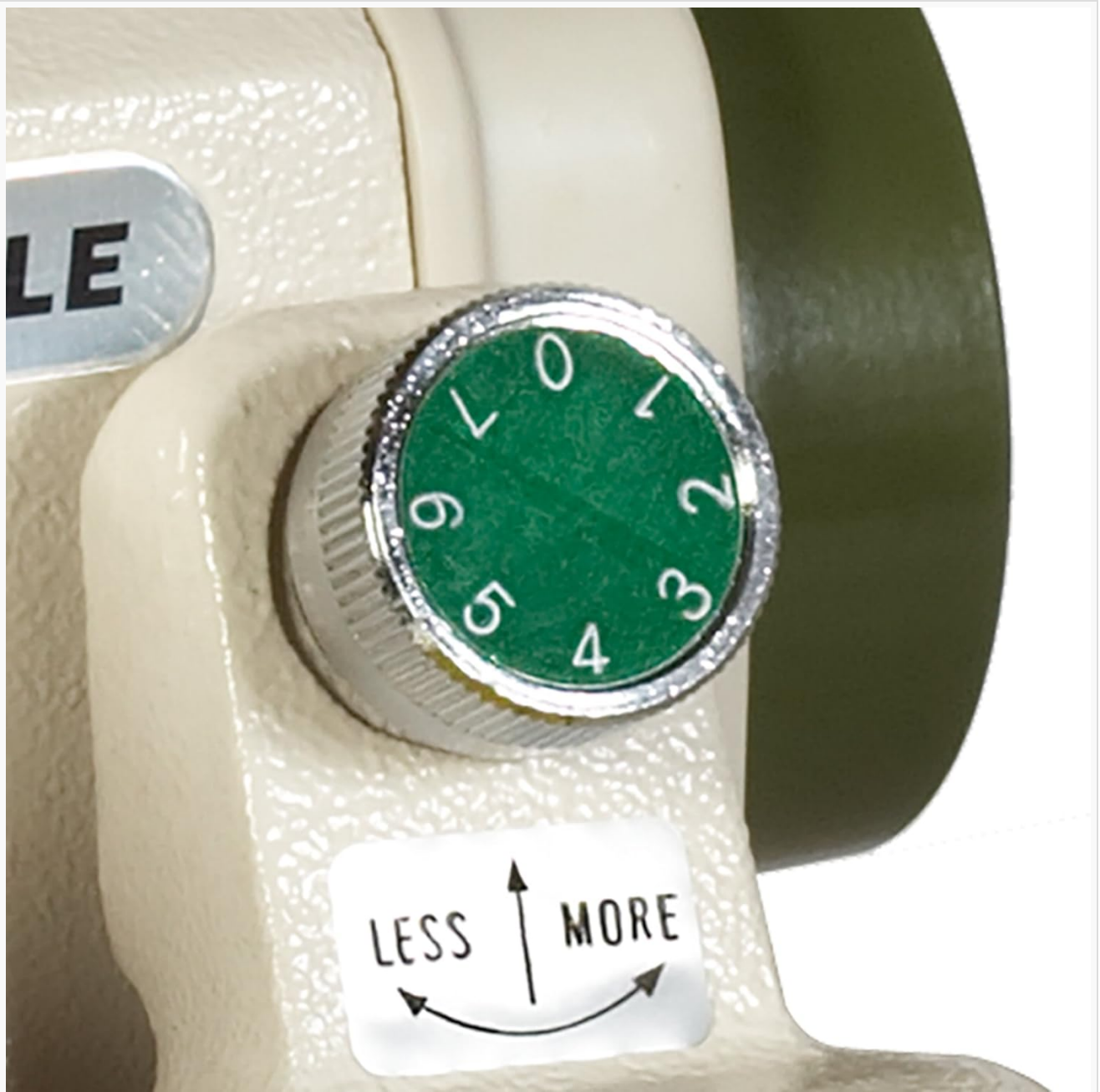
Figure 5.2: Close-up of the stitch penetration adjustment dial. This dial allows precise control over the depth of the needle's penetration into the fabric.
