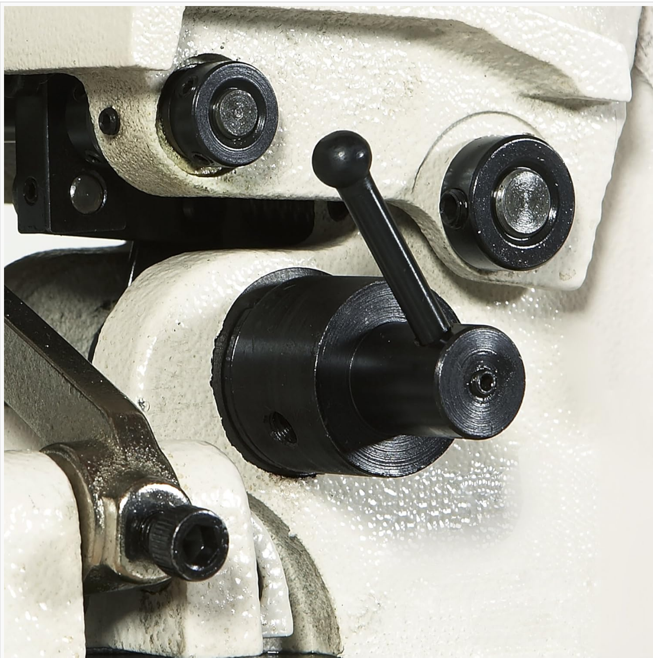
Figure 5.1: Close-up view of the knee-activated frame drop lever. This lever allows for quick and easy fabric positioning.
