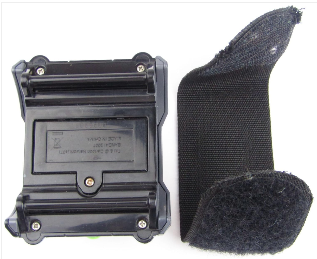
Figure 2: Underside view of the Omnitrix, indicating the location of the battery compartment screws.
