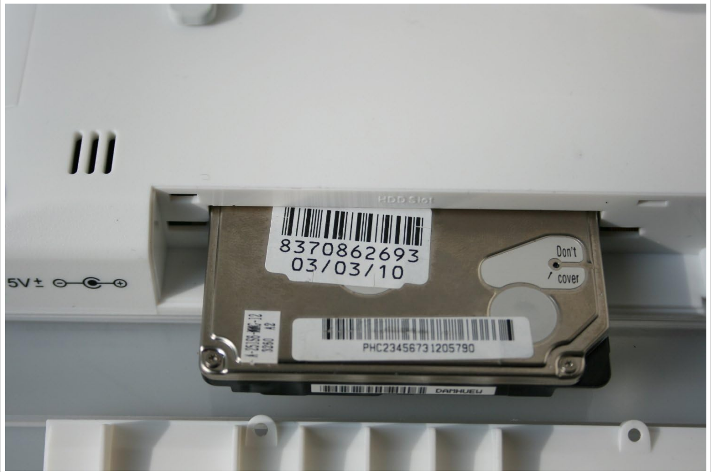
Figure 4.3: HDD Slot. This image shows a close-up of the HDD slot located on the back of the digital photo frame, with a hard drive inserted. The hard drive shown has a serial number PHC23456731205790. This slot allows for expanded storage capacity.
