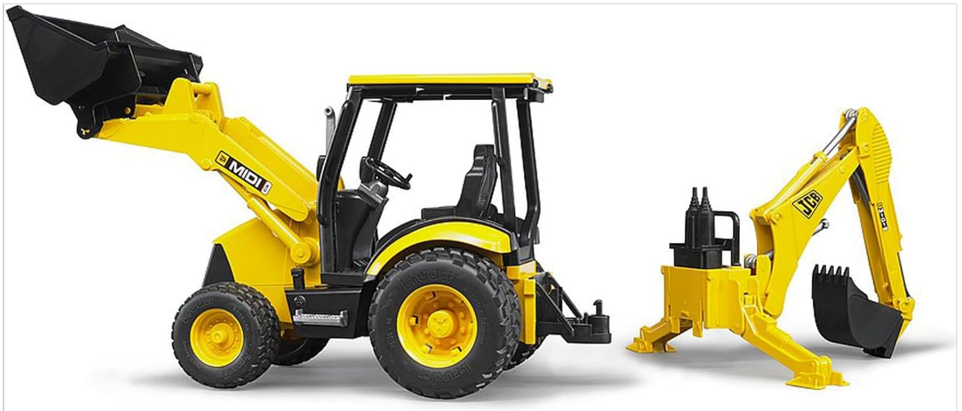
Image: The backhoe loader with the rear shovel detached, illustrating its modular design.
