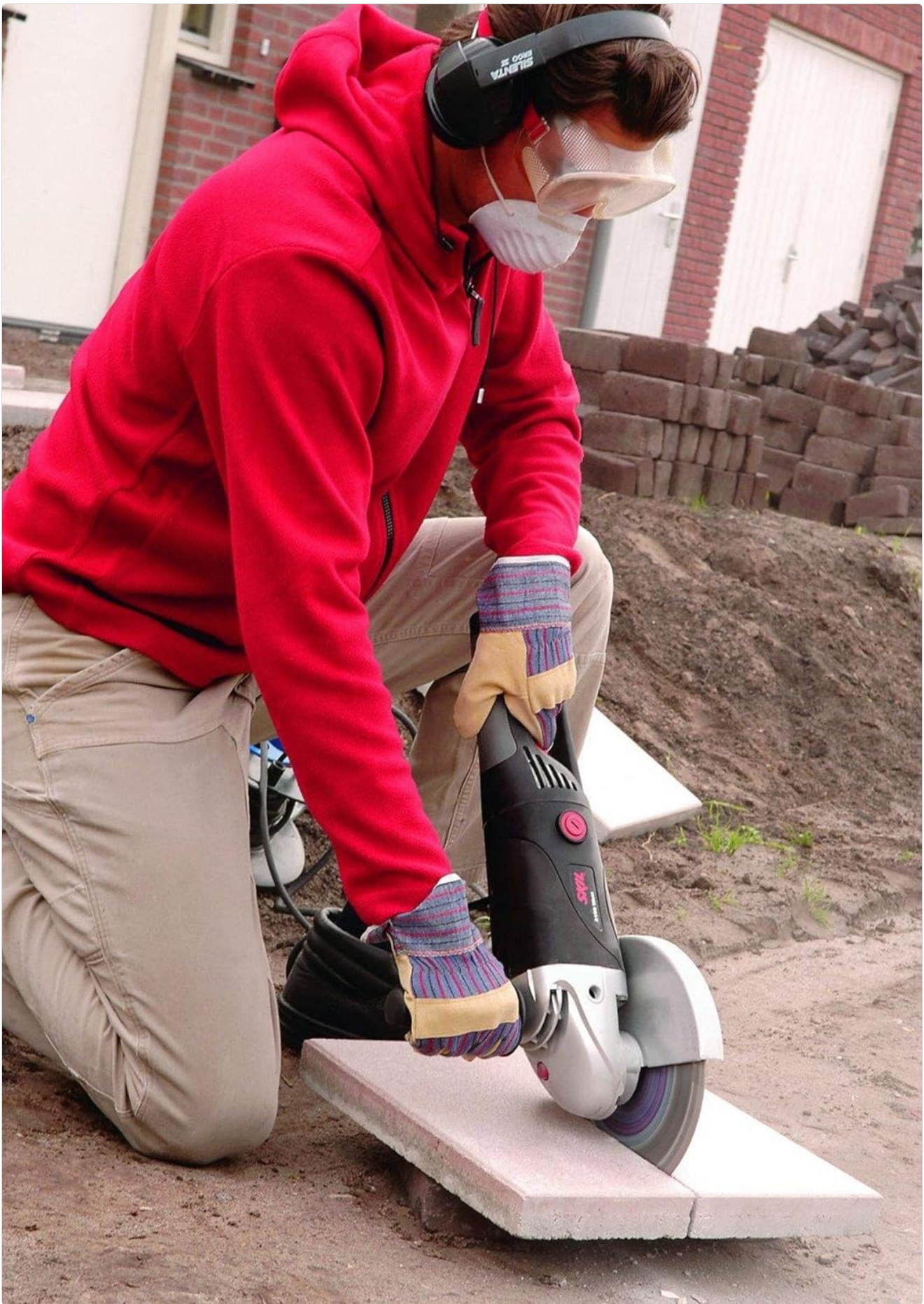
Image 3.1: A person wearing safety glasses, ear protection, and a dust mask, using the Skil angle grinder to cut a concrete slab. The grinder is held firmly, and sparks are visible, indicating active cutting.
