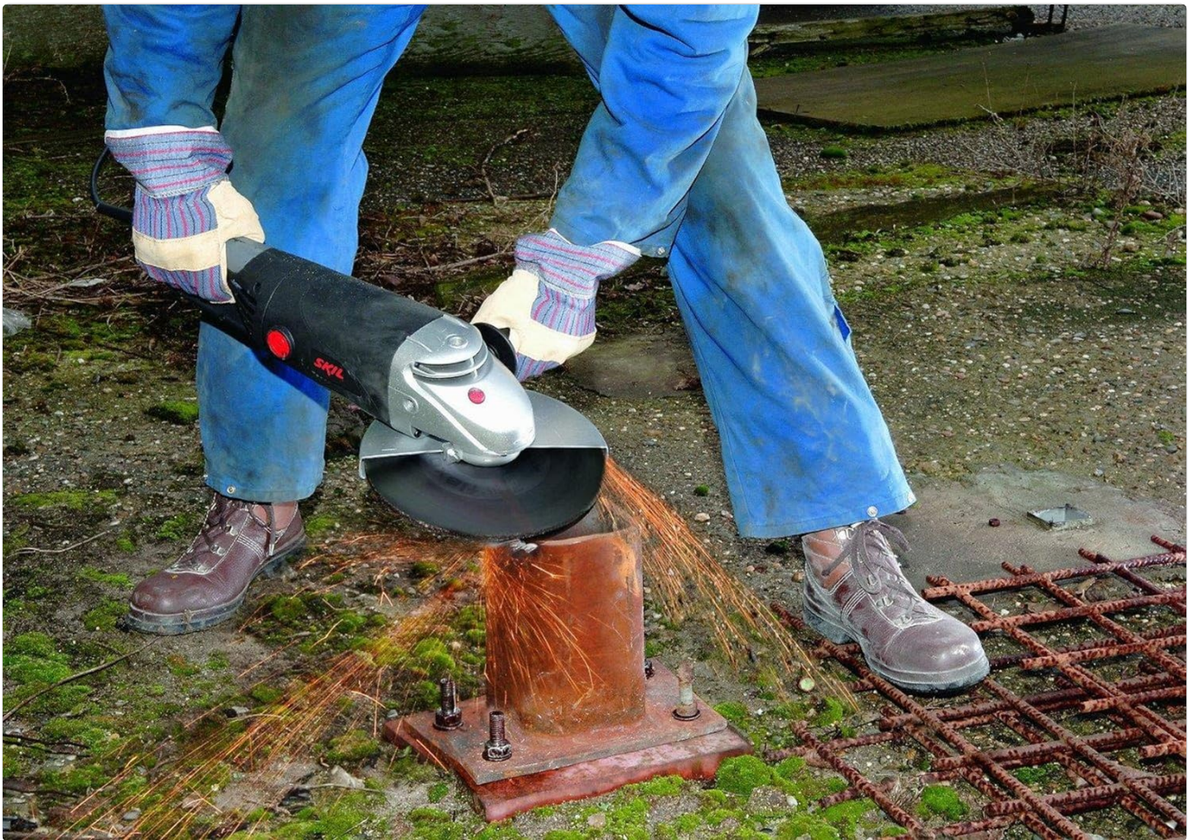
Image 3.2: A person operating the Skil angle grinder to cut a metal pipe, producing a shower of sparks. The operator is wearing protective gloves, and the tool is held securely with both hands.
