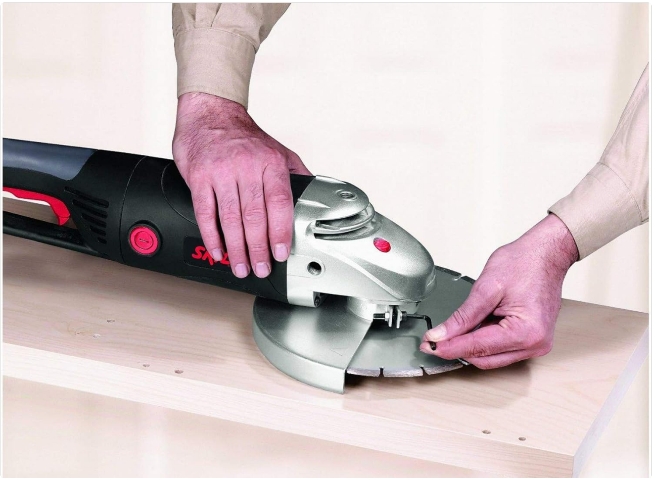
Image 2.1: Close-up view of hands demonstrating the process of changing a grinding disc on the Skil angle grinder. An accessory key is used to loosen the clamping nut while the spindle lock is engaged.
