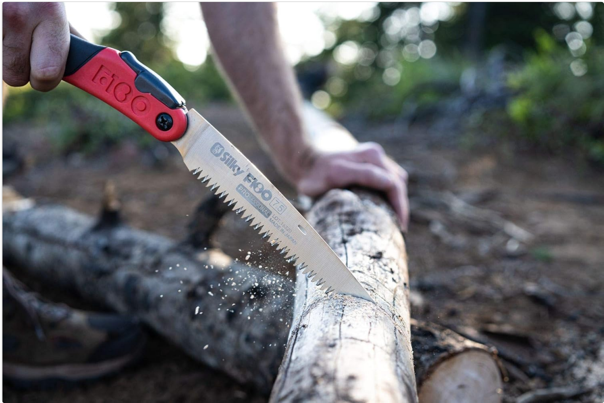
Image 4.2: A user demonstrating the proper technique for cutting a log with the Silky F180 Folding Saw, emphasizing the pull stroke.
