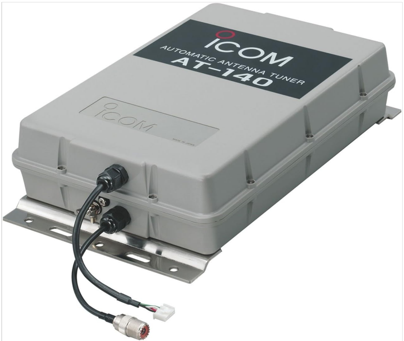
Image: The Icom AT-140 Automatic Antenna Tuner, a grey rectangular unit with "ICOM AUTOMATIC ANTENNA TUNER AT-140" printed on top. Two black cables are connected to its side, leading to a PL-259 connector and a multi-pin connector, indicating its readiness for installation.
