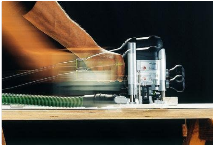
The image captures the Festool OF 1010 EBQ Router in operation, with motion blur indicating active use and the dust extraction system effectively managing debris.
