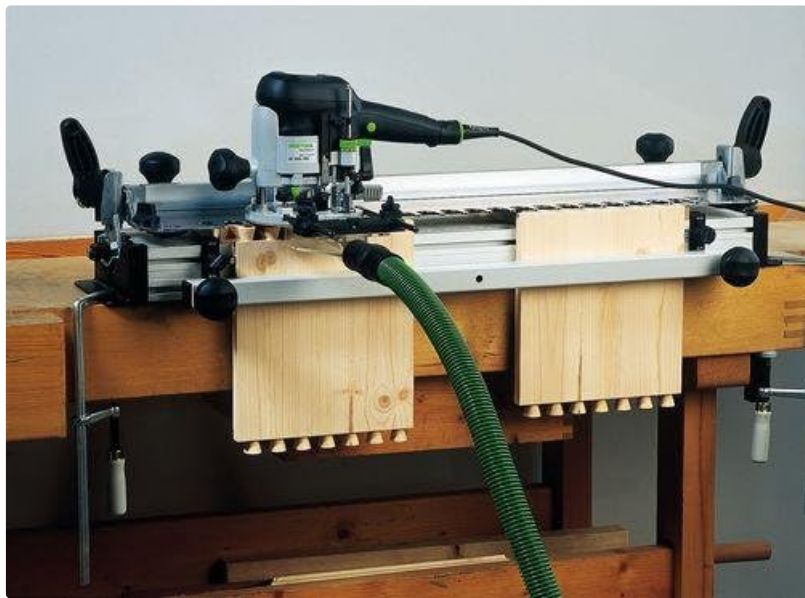
This image shows the Festool OF 1010 EBQ Router integrated with a dovetail jig, illustrating its application in creating precise woodworking joints.
