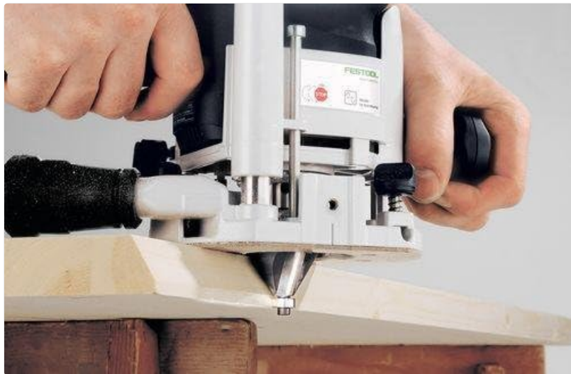
This close-up view illustrates the Festool OF 1010 EBQ Router actively shaping the edge of a wooden board, highlighting its precision in profiling.
