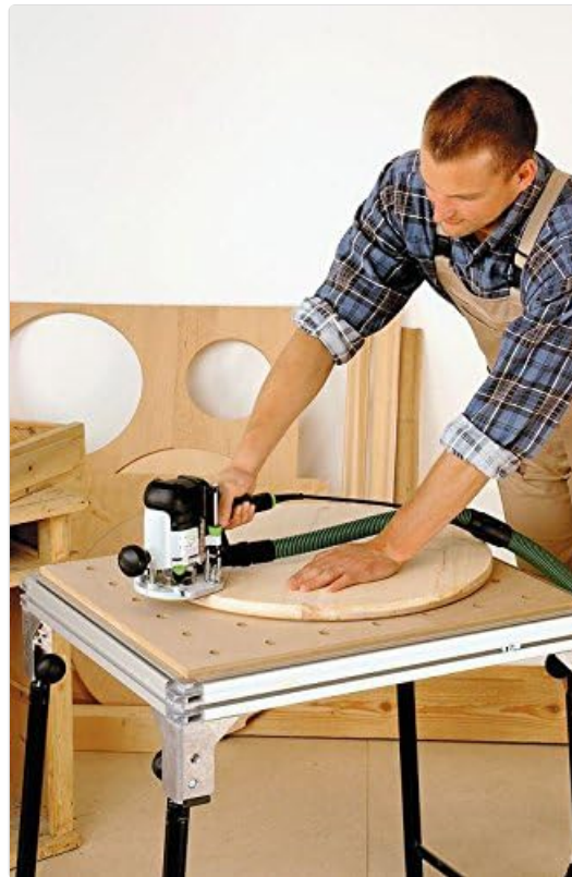
A user is demonstrating the Festool OF 1010 EBQ Router's capability to create circular cuts on a wooden panel, likely using a circle routing jig.
