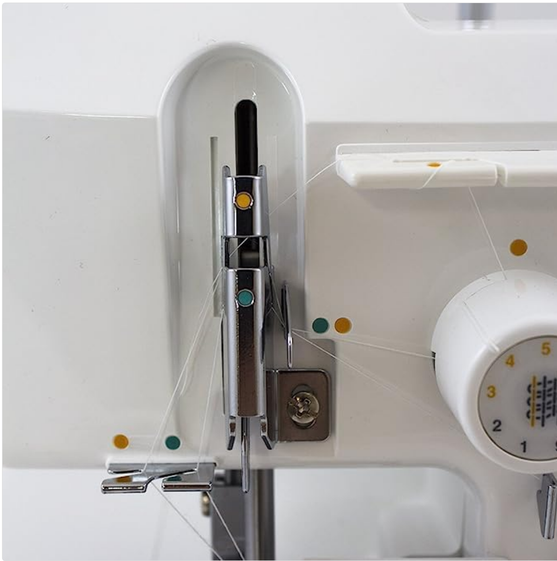
Figure 3.4.2: Detailed view of the looper area on the JUKI MO644D, showing the intricate threading paths for the lower and upper loopers.
