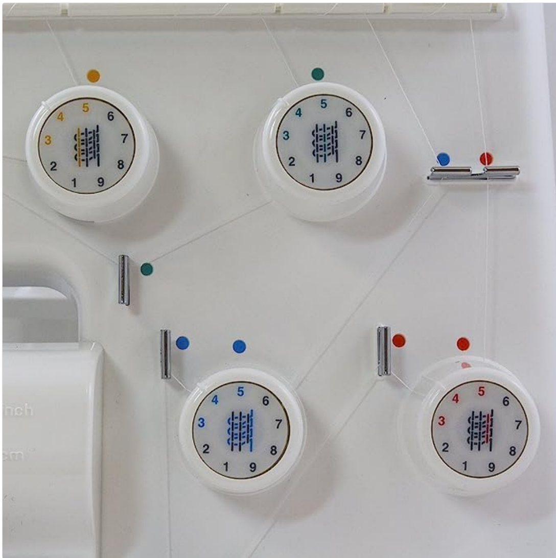
Figure 3.4.1: Close-up view of the color-coded tension dials on the JUKI MO644D, indicating the threading path for each thread.
