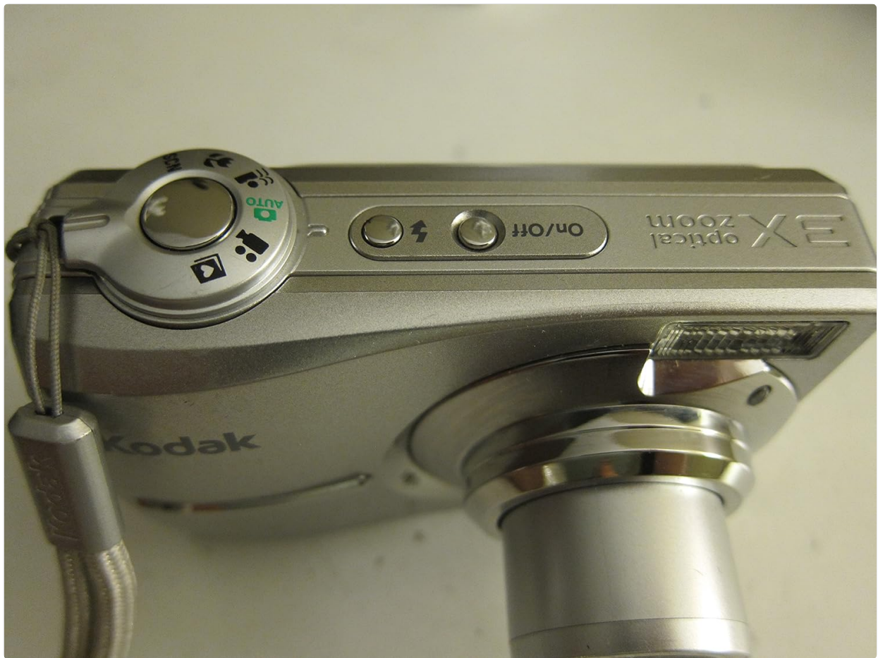
Figure 3.1: Top view of the camera, highlighting the power button and mode dial.
