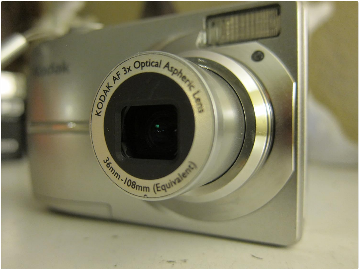
Figure 3.3: Angled front view of the camera with the lens extended, demonstrating optical zoom.
