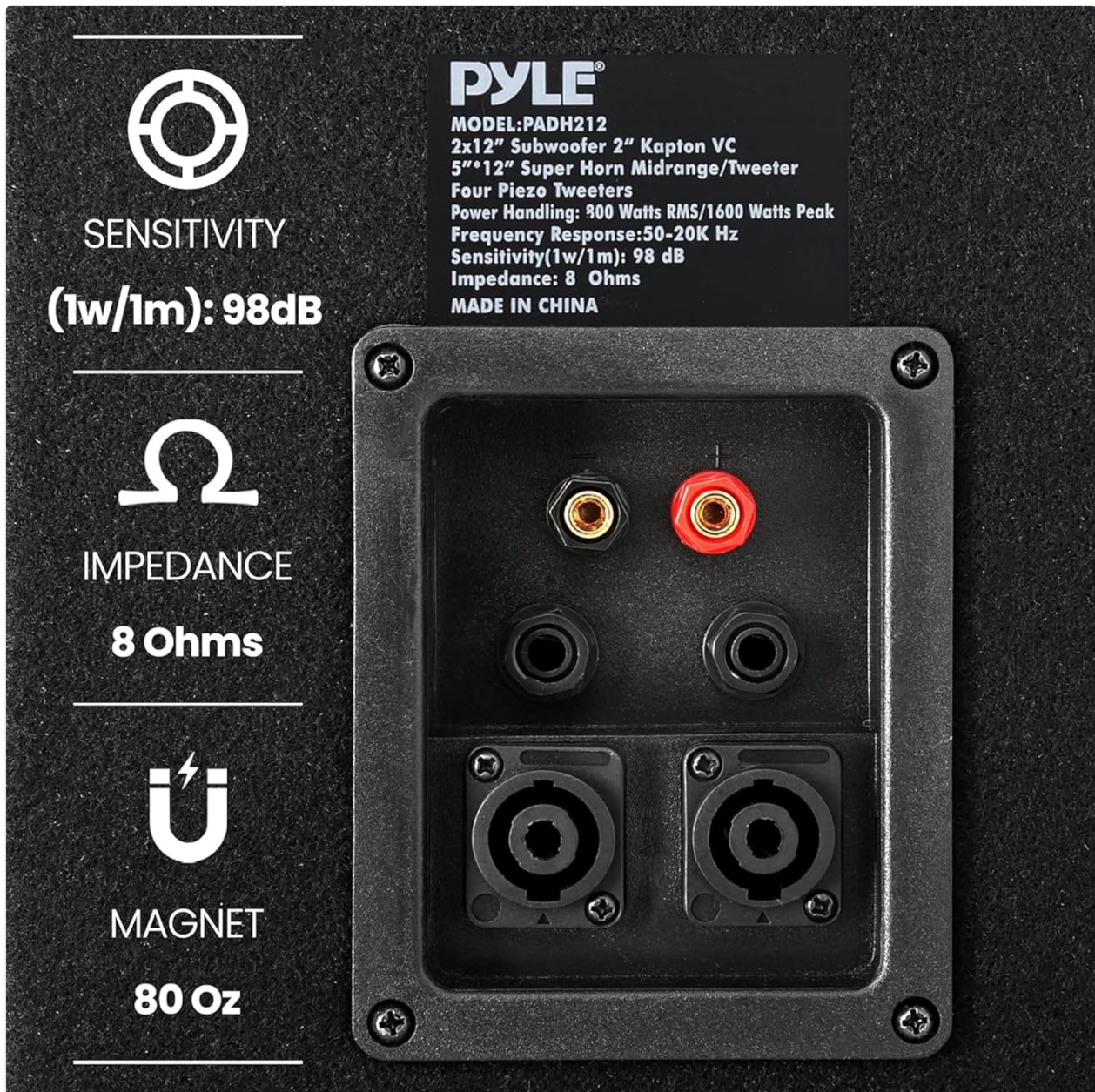
Figure 6: Rear Connection Panel. The rear panel of the Pyle PADH212 speaker, displaying the various input terminals including Speakon and binding posts, along with a label listing technical specifications such as sensitivity, impedance, and magnet size.
