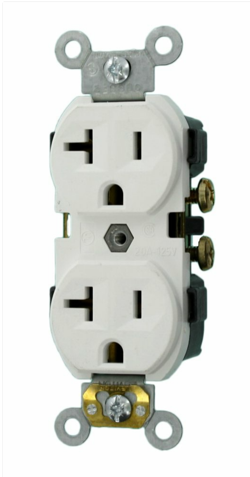
Image 1.1: Front view of the Leviton CR20-W 20-Amp, 125-Volt Commercial Grade Duplex Receptacle in White. This image displays the two standard NEMA 5-20R outlets, the mounting strap, and the terminal screws on the side.
