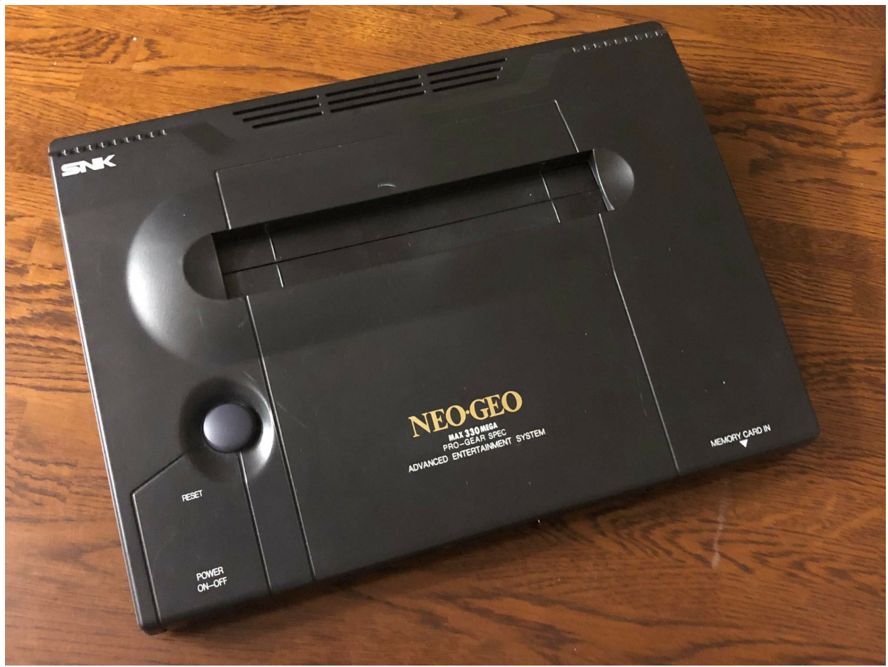
Image 2.1: Neo Geo AES console detail. This image provides a closer look at the console's top surface, highlighting the large cartridge slot, the 'POWER ON-OFF' switch, and the 'RESET' button. The 'MEMORY CARD IN' slot is also visible.
