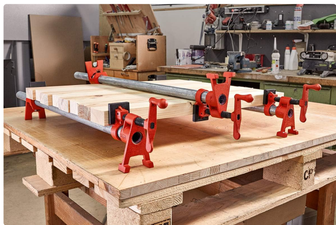
Image 2: BESSEY BPC-H34 pipe clamps securing multiple wood pieces for a glue-up project on a workbench, demonstrating their stability and application.
