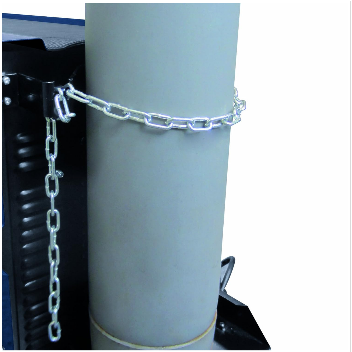
Image: A robust metal chain securely fastening a gas bottle to the side of the welding machine, ensuring stability and safety during operation and transport.
