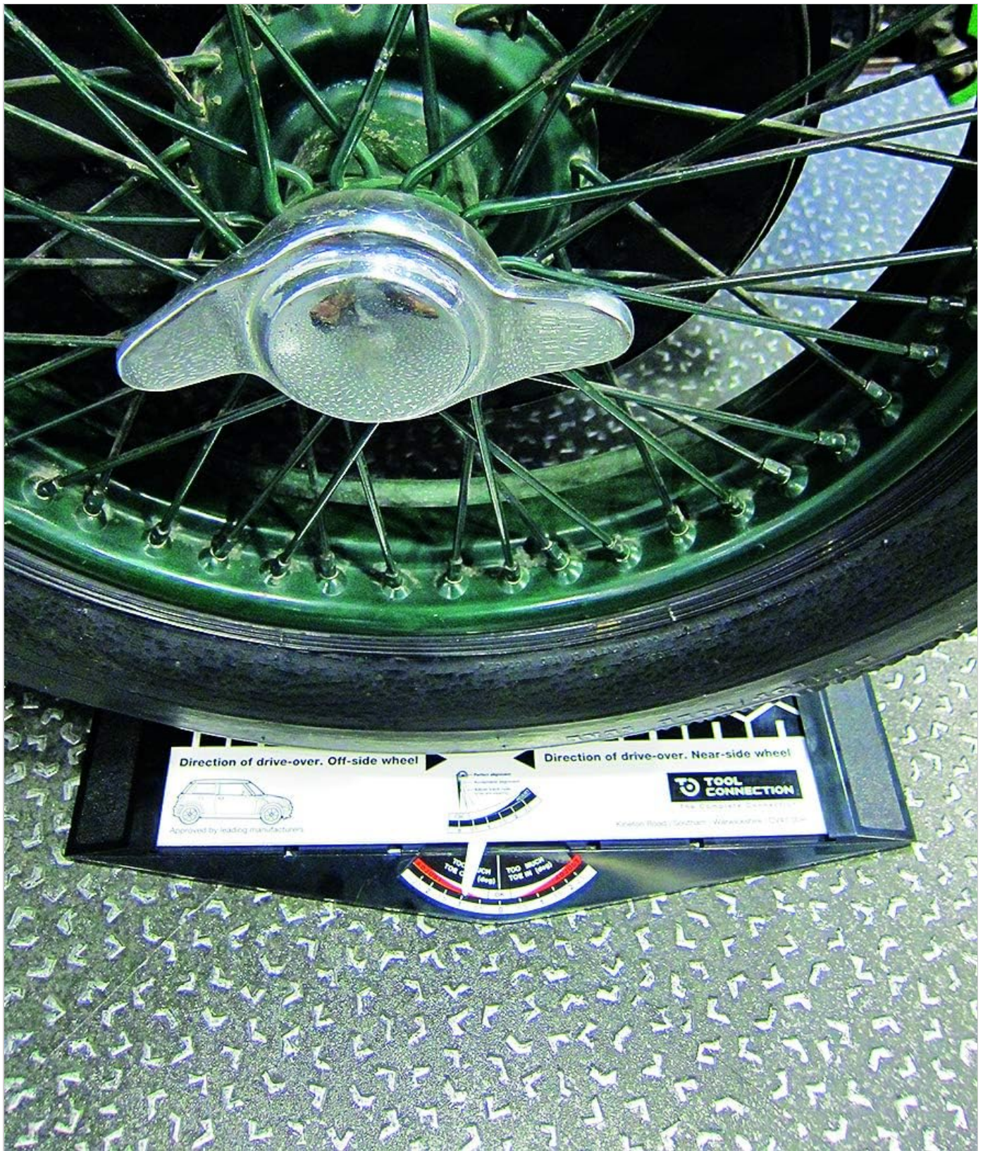
Figure 3: The Trakrite gauge being used with a classic car, demonstrating its versatility across different vehicle types. The wheel is centered over the gauge for an accurate reading.
