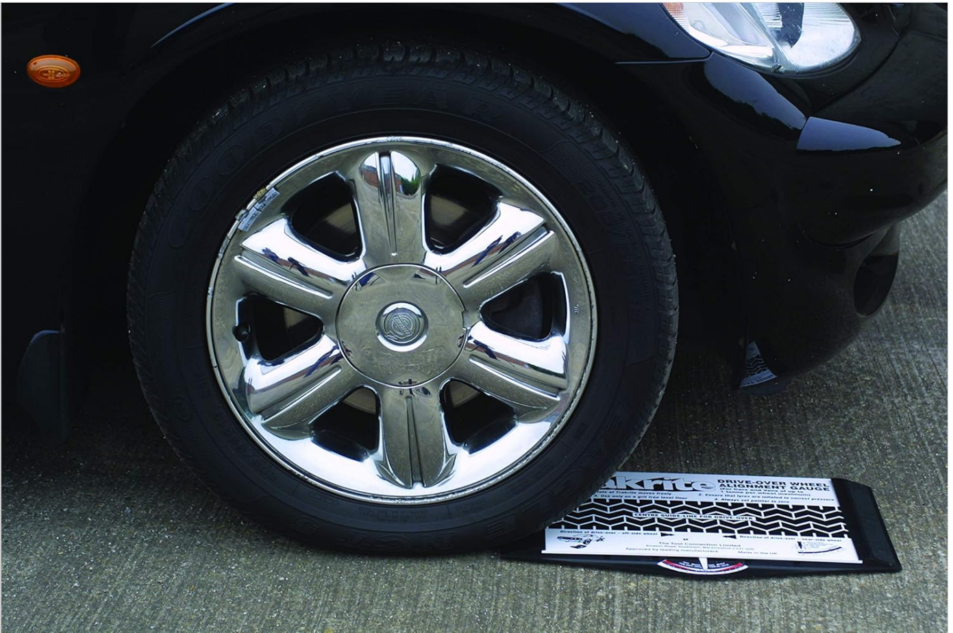
Figure 2: A vehicle's front wheel positioned on the Trakrite gauge, ready for an alignment check. The gauge is placed directly in the path of the wheel.
