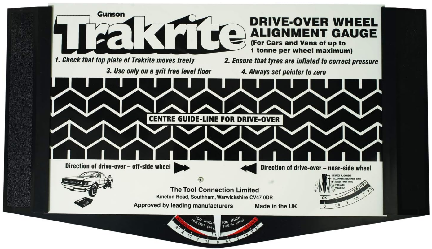
Figure 1: The Trakrite gauge showing key setup instructions printed on its surface. These include checking plate movement, ensuring correct tire pressure, using a grit-free floor, and zeroing the pointer.
