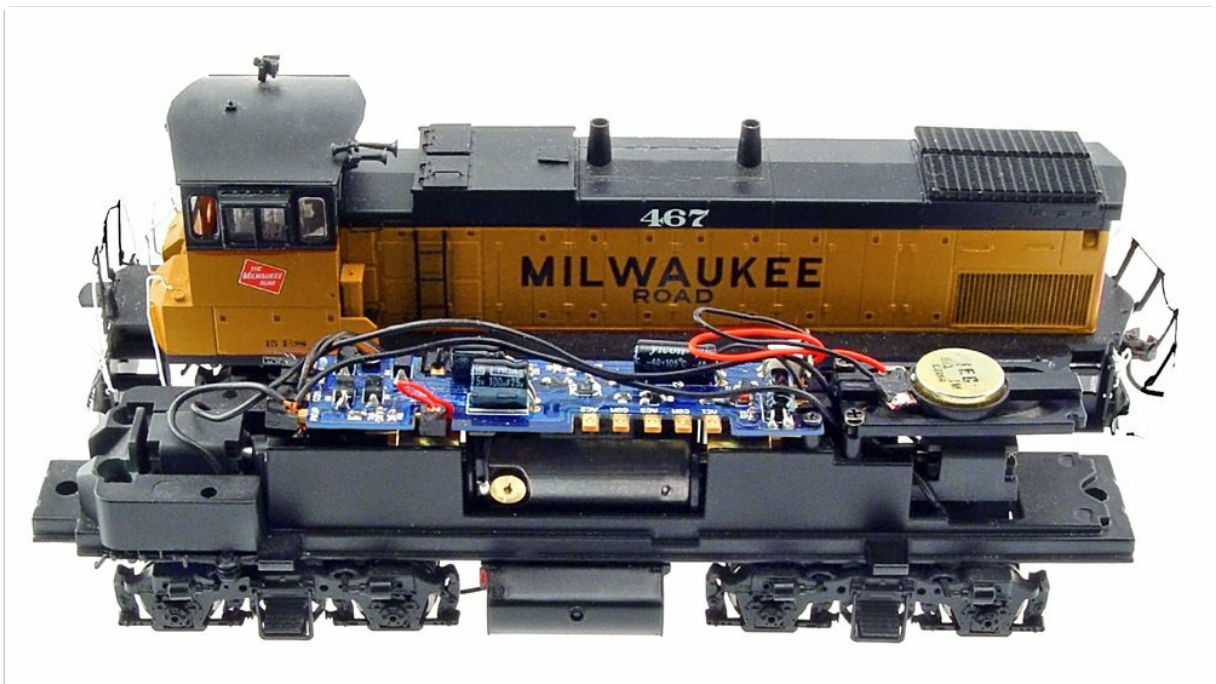
Image showing the MRC HO Drop-in Sound Decoder, a compact electronic board with various components and a speaker connection. This decoder is designed to replace the original circuit board in Athearn MP15 locomotives.
