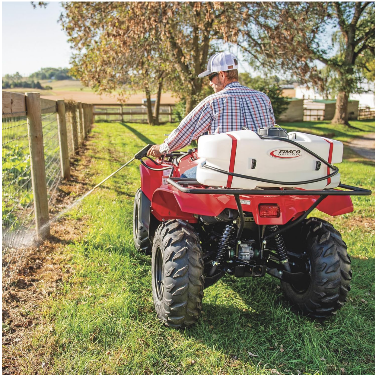
Figure 4.1: Fimco 25 Gallon Spot Sprayer mounted on an ATV. This image demonstrates how the sprayer can be securely placed on the rear rack of an ATV for mobile spraying operations.
