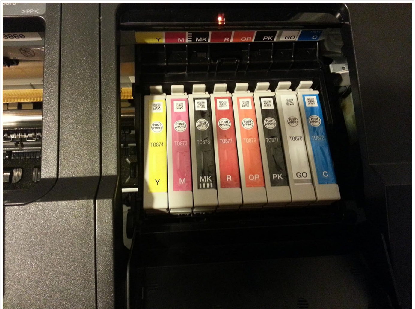
Figure 3: A close-up view of the Epson UltraChrome Hi-Gloss 2 ink cartridges, showing their individual colors and labels, installed within the printer's ink bay.
