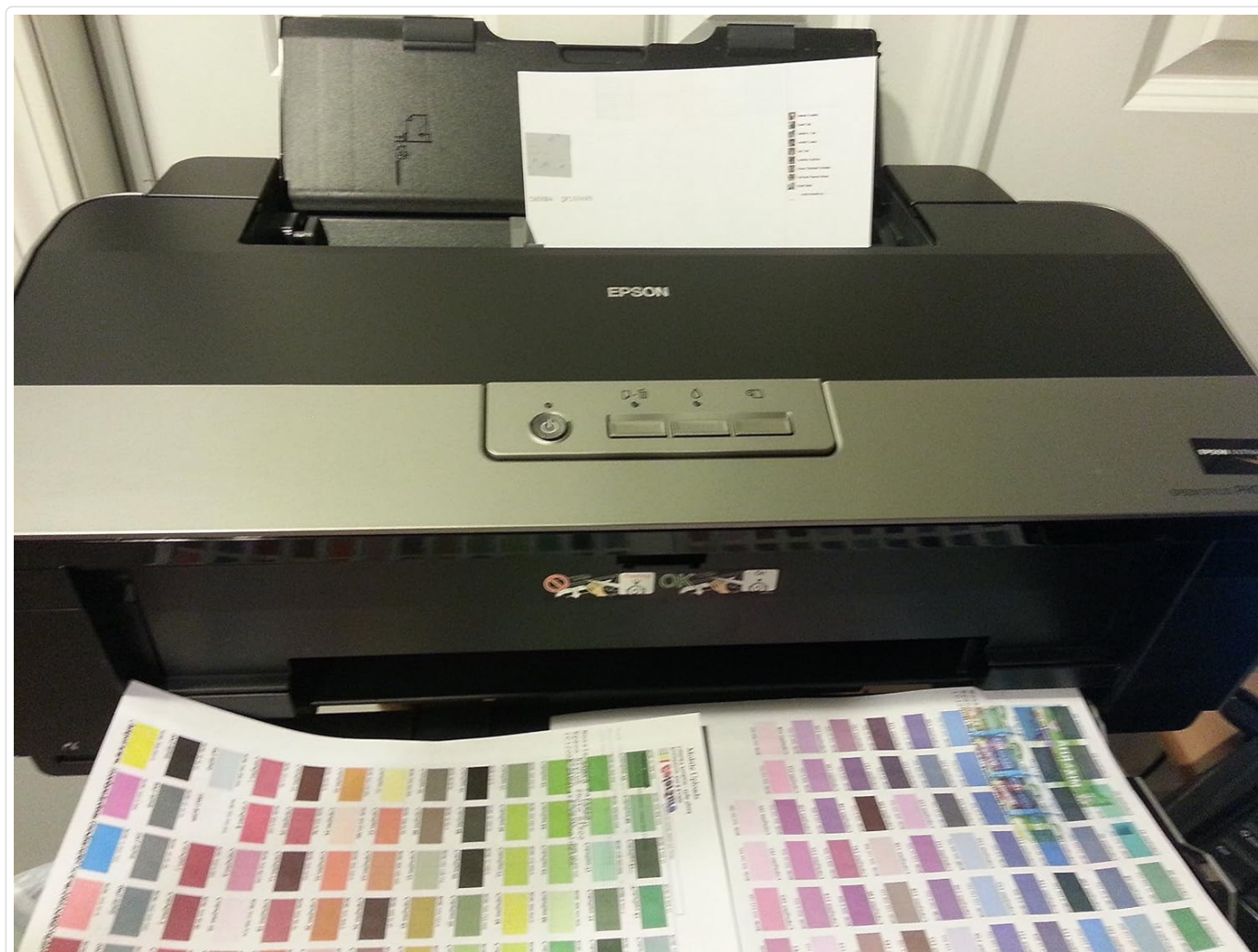
Figure 1: The Epson Stylus Photo R1900 printer with paper loaded in the top feeder and a color calibration sheet exiting the front.
