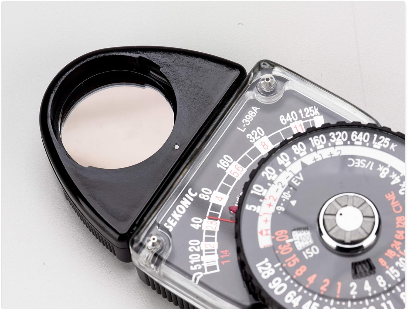
Figure 4.1: Detail of the exposure dial, highlighting the ISO setting area.
