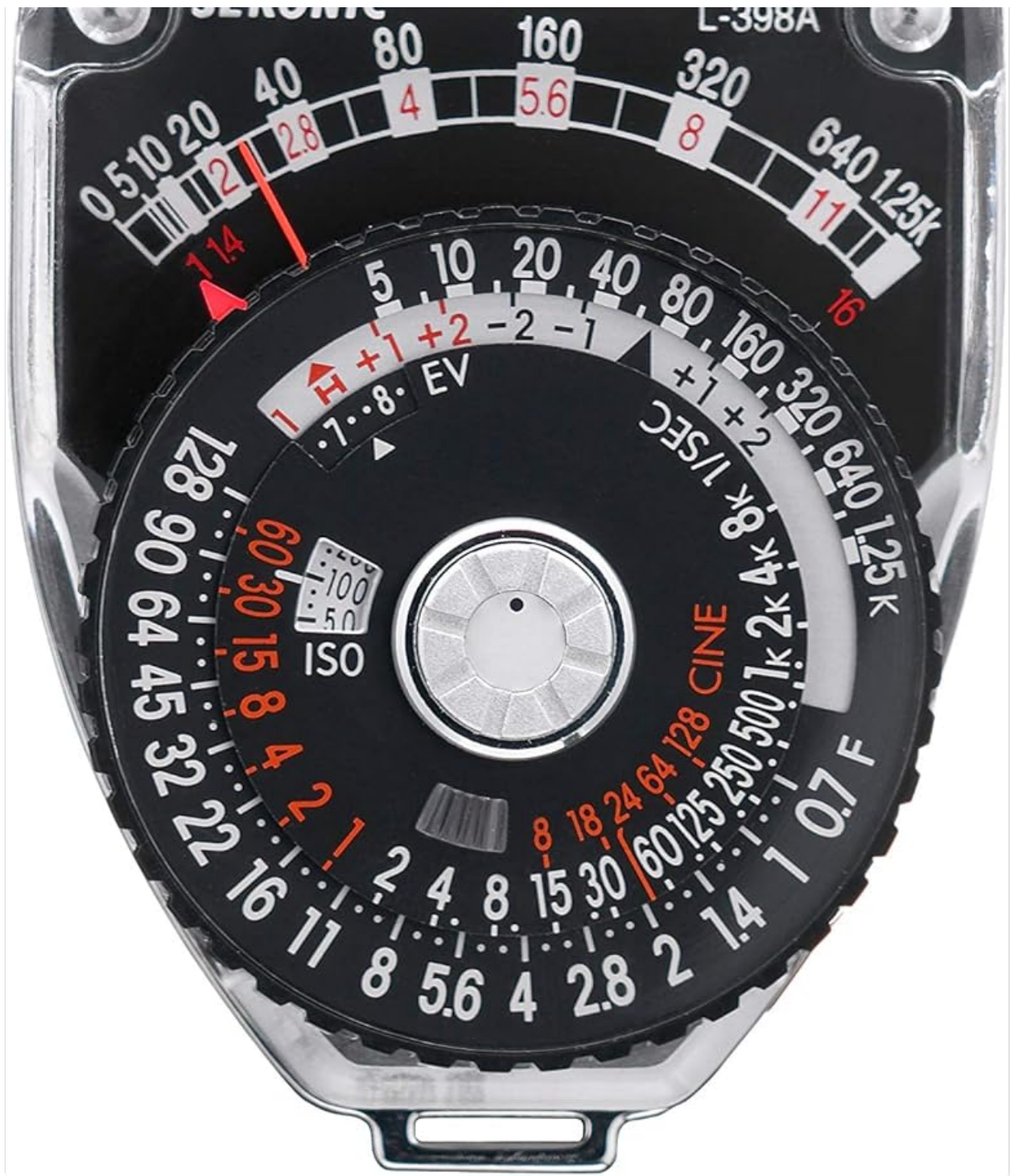
Figure 1.1: Front view of the Sekonic L-398A Light Meter Studio Deluxe III, showing the Lumisphere and the exposure dial.
