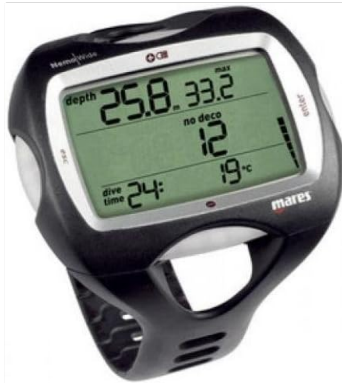
Figure 1: The Mares Nemo Wide 2 Dive Computer. The display shows current depth (25.8), maximum depth (33.2), no-decompression limit (12 minutes), dive time (24 minutes), and water temperature (19°C). The device has four buttons for navigation and settings.
