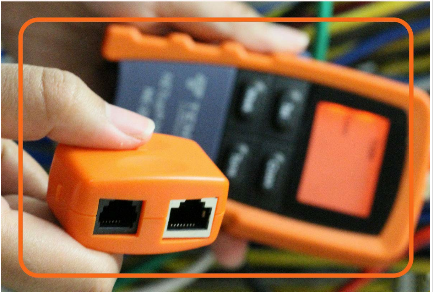
The NC-100 main unit and its remote test unit, demonstrating the setup for generating digital tone patterns for cable tracing.
