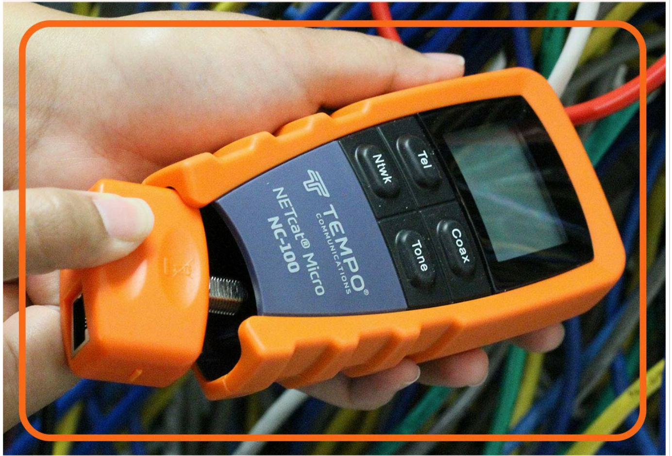
A hand connecting a coaxial cable to the Tempo Communications NC-100, demonstrating its capability to test various cable types.
