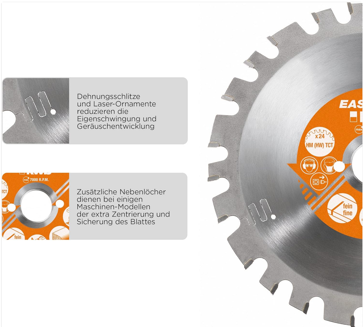
Figure 7: Close-up of the blade illustrating expansion slots and laser ornaments designed to reduce vibration and noise, along with additional holes for extra centering and securing on certain machine models.
