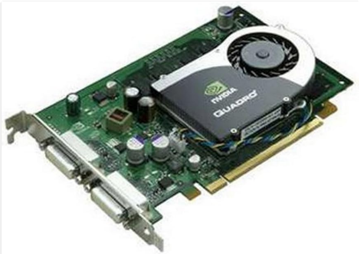
Image 1.1: The HP NVIDIA Quadro FX570 256MB PCIe Graphics Card. This image displays the green circuit board, the NVIDIA Quadro branded heatsink and fan assembly, and the dual DVI output ports.
