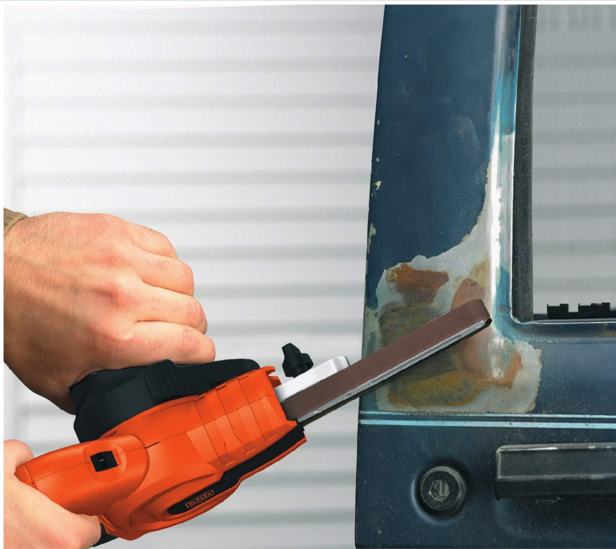
Figure 4: Sanding a car door frame, illustrating the tool's ability to access narrow and curved areas for surface preparation.
