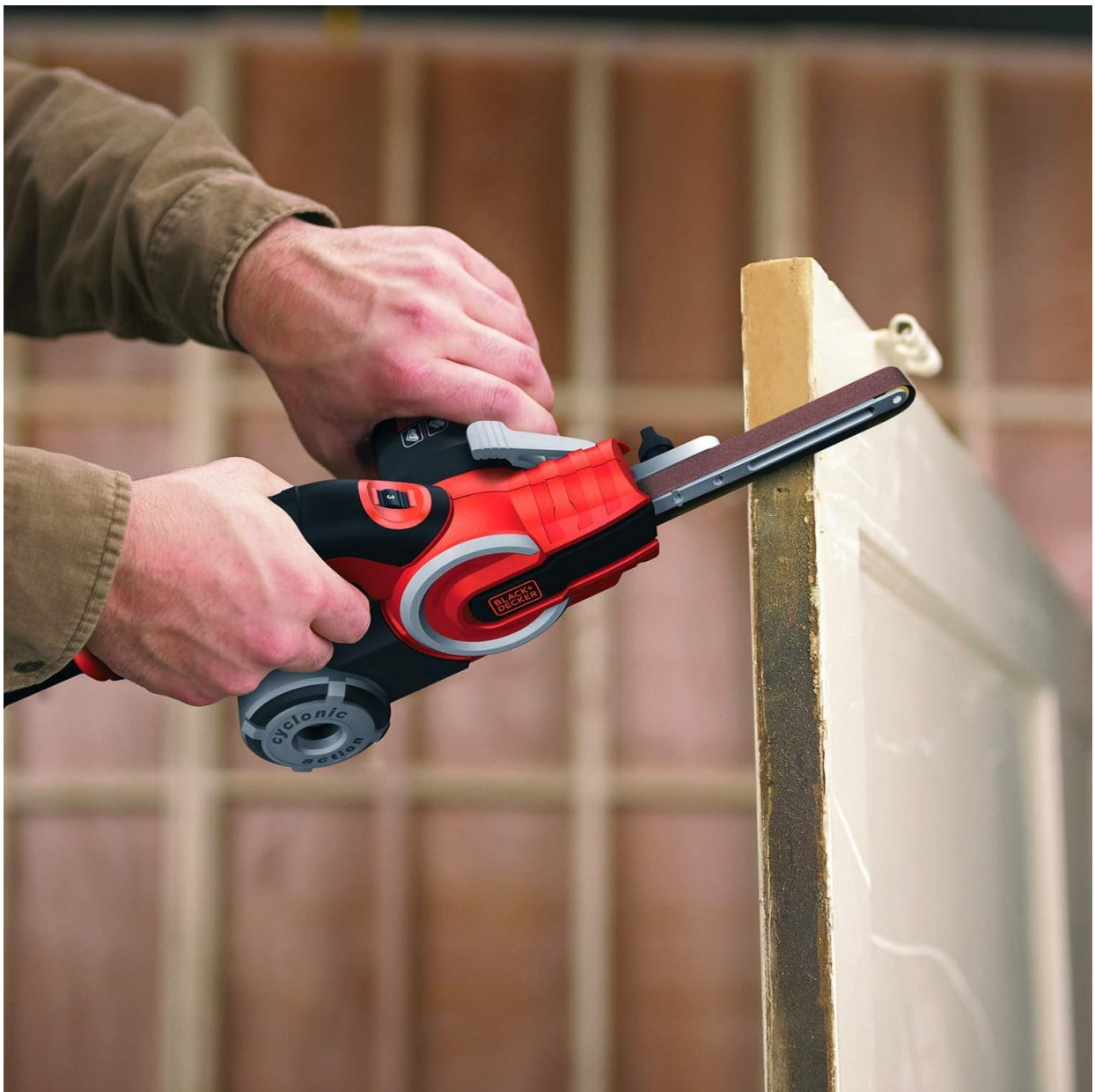
Figure 6: The power file sander being used on a wooden frame, demonstrating its utility for preparing wood surfaces.
