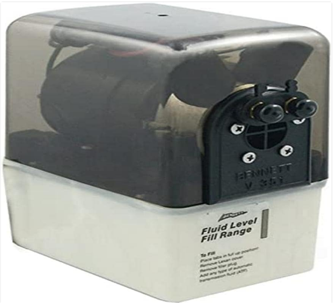
Figure 1: Bennett V351HPU1 Hydraulic Power Unit. This image displays the Bennett V351HPU1 Hydraulic Power Unit. It features a translucent Lexan cover, allowing visual inspection of internal components and fluid levels. The lower section is a white reservoir with a 'Fluid Level Fill Range' indicator. The unit's compact design is evident, with the motor and solenoid valves visible under the cover.
