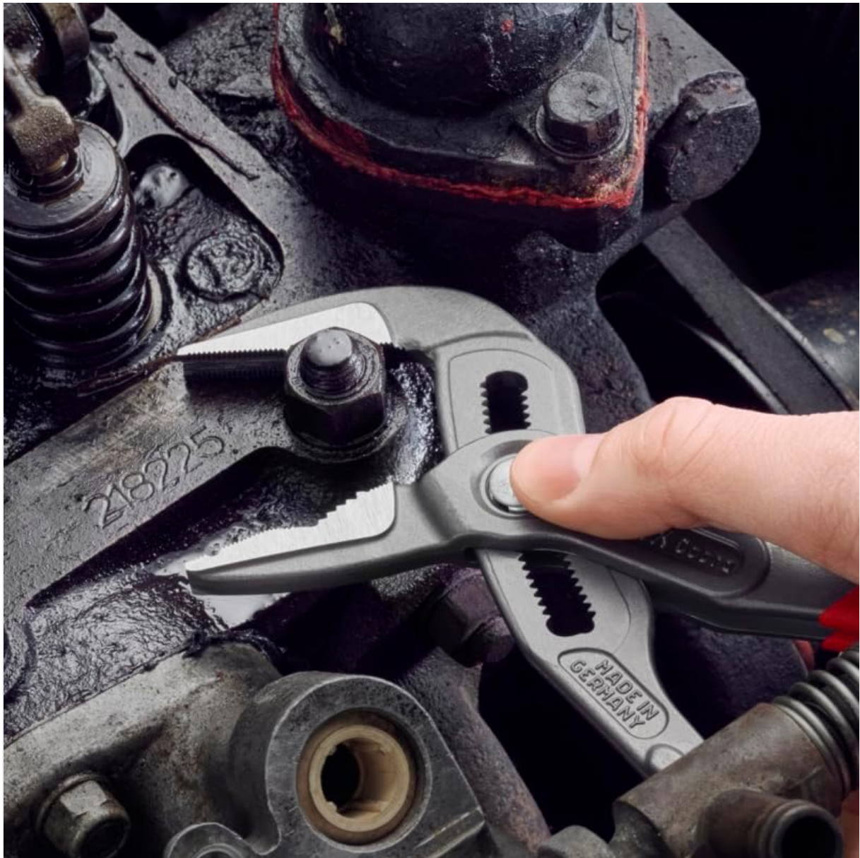
Figure 4.1: Detail of the push-button for quick and precise jaw adjustment.
