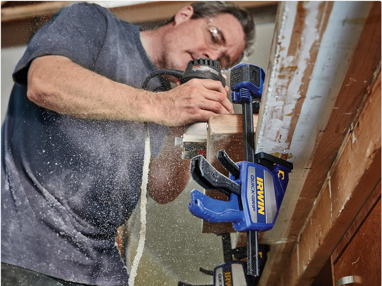
Figure 4: Clamp configured for spreading. This image illustrates the IRWIN QUICK-GRIP XP clamp being used to push apart two wooden pieces, demonstrating its spreading functionality.
