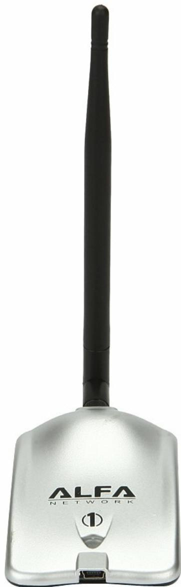
Figure 1: Front view of the ALFA Network AWUS036H adapter with the 5dBi antenna connected. The USB port is visible at the bottom.
