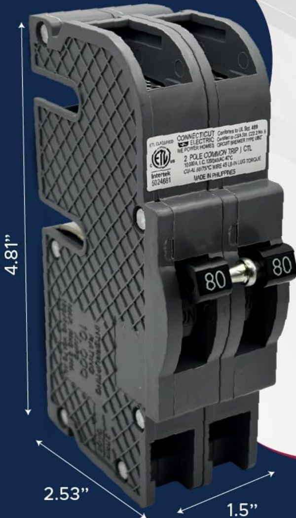
Image 1.1: Front view of the Connecticut Electric UBIZ280 circuit breaker, showing its dimensions (4.81" height, 2.53" depth, 1.5" width) and key specifications like 80 Amp, 2 Pole, 120/240 Volt, UL 489 Compliant, and ETL Listed. It is compatible with Zinsco load centers.
