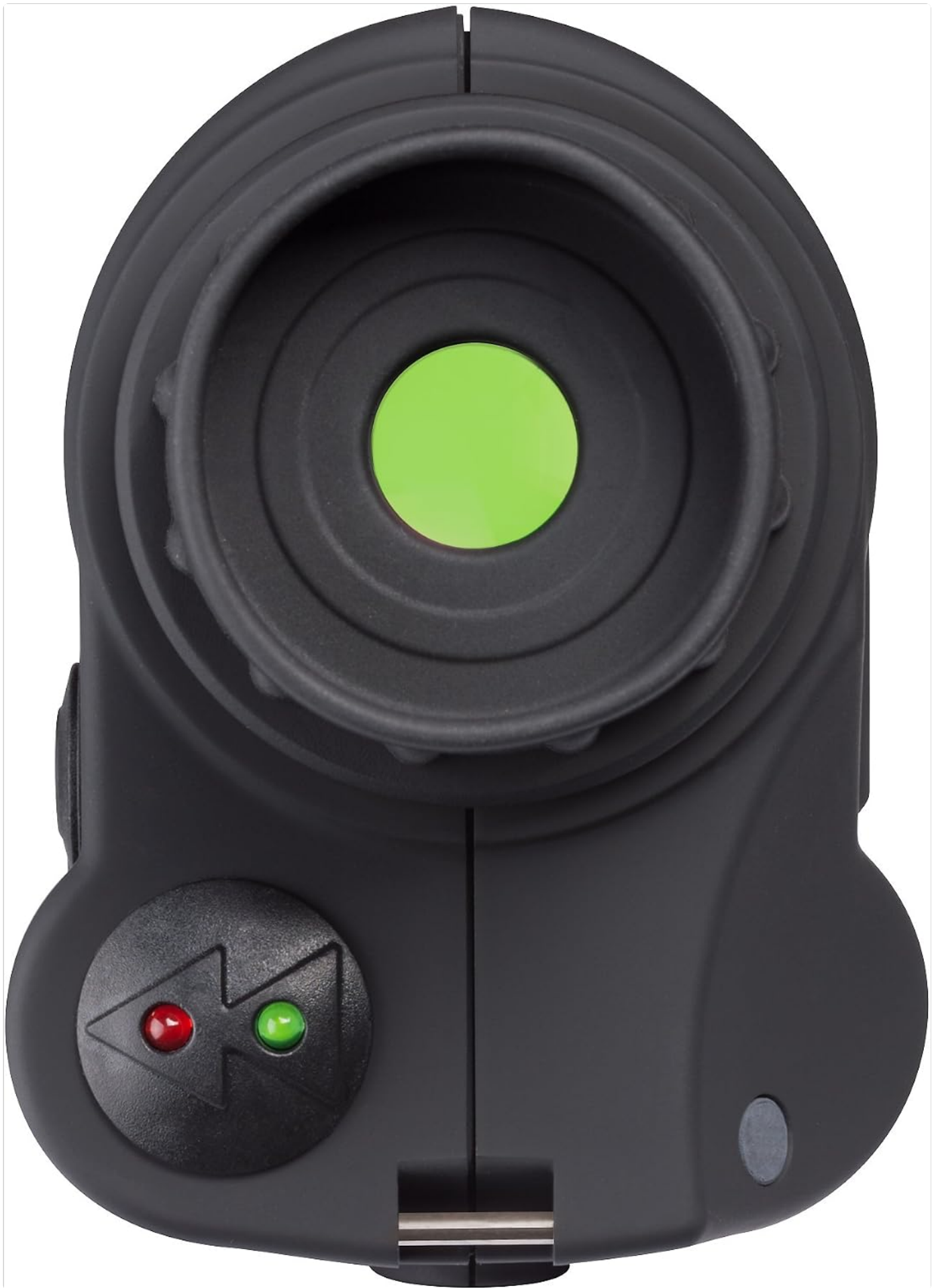
Figure 4.3: Close-up view of the eyepiece, showing the green image intensifier tube.
