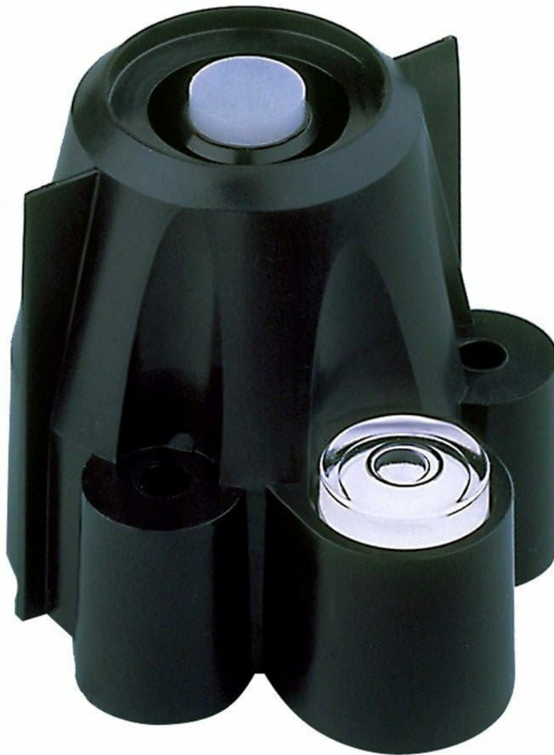
Figure 1: The Davis Instruments 6450 Solar Radiation Sensor. This black plastic unit features a translucent white dome for light detection and a clear bubble level for precise horizontal alignment during installation.
