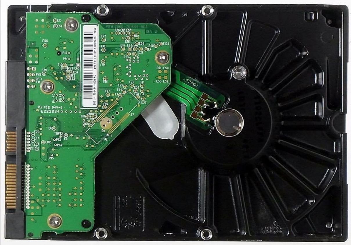
Image 3: Bottom view of the WD Blue 160 GB PATA hard drive, revealing the green printed circuit board (PCB) and the motor assembly. This view shows the electronic components responsible for drive operation.
