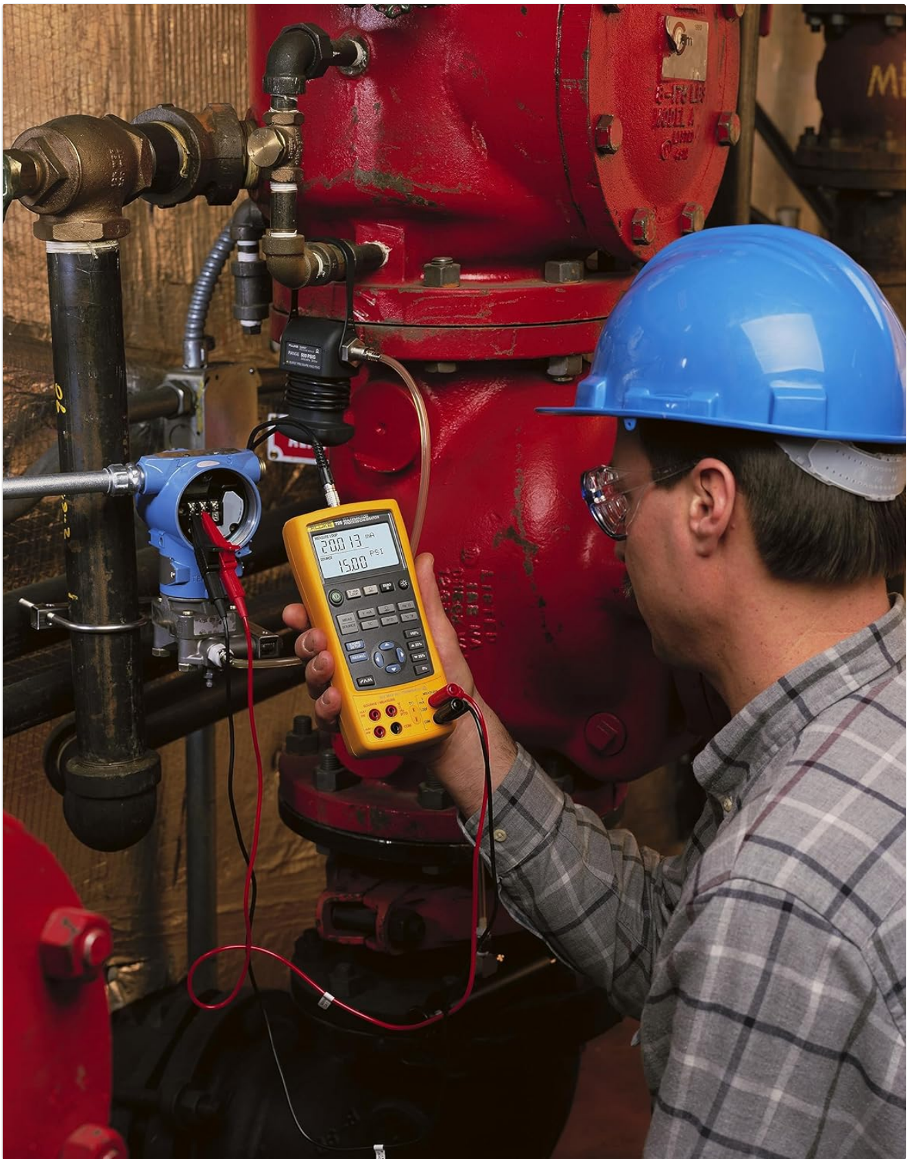
Figure 3: The Fluke 725 calibrator connected to a pressure transmitter, demonstrating its application in process calibration.
