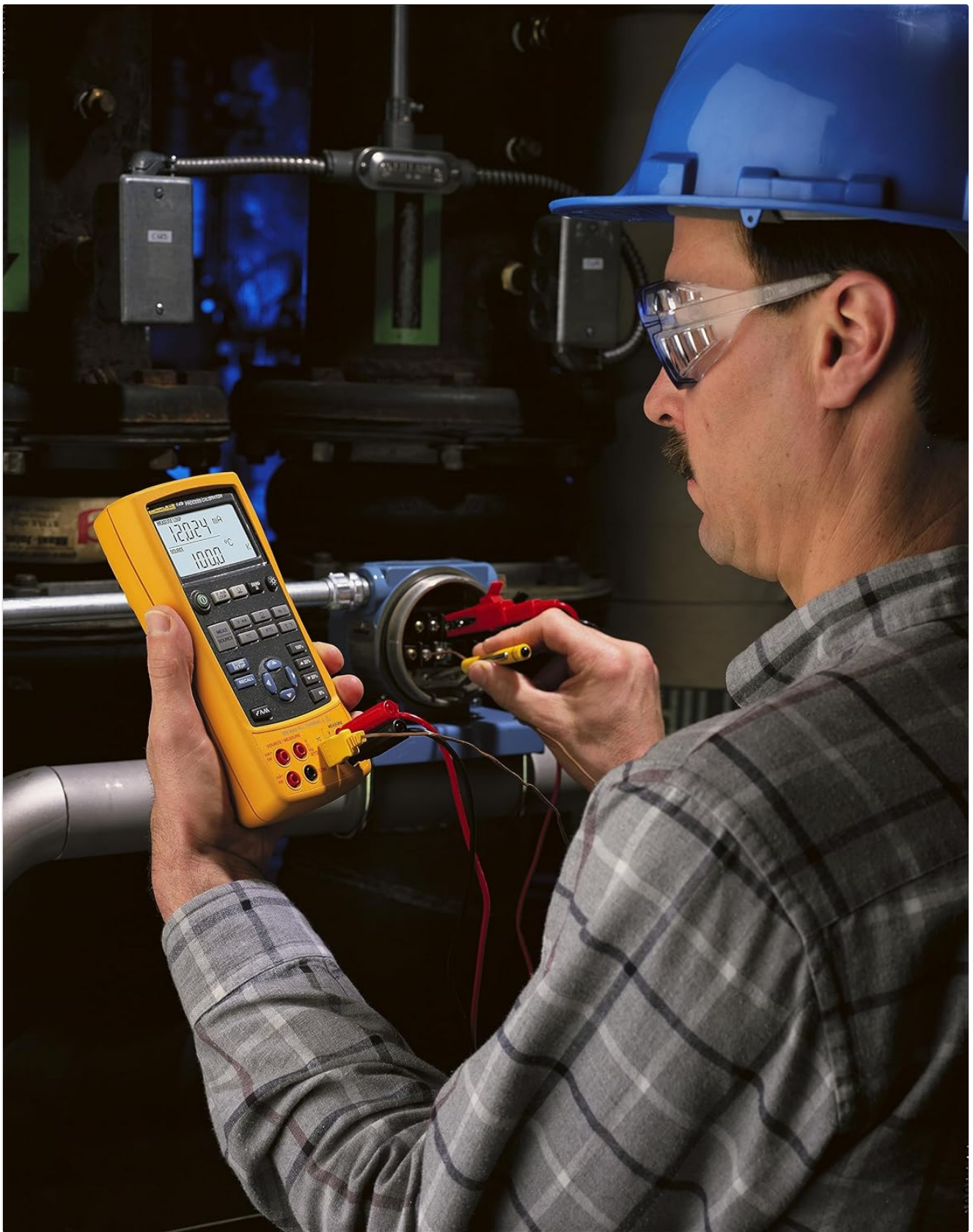
Figure 2: A technician utilizing the Fluke 725 to connect and calibrate industrial process equipment.
