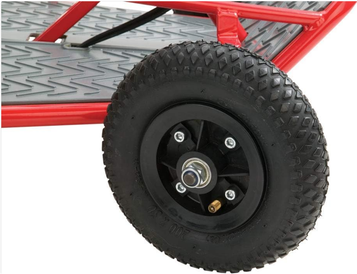
Figure 6: Close-up of the knobby pneumatic tire for enhanced traction.
