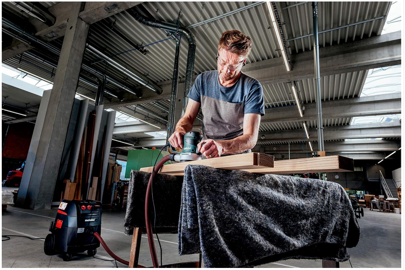
Figure 3.2: The sander in use with an external dust extraction system, demonstrating efficient dust collection during operation.
