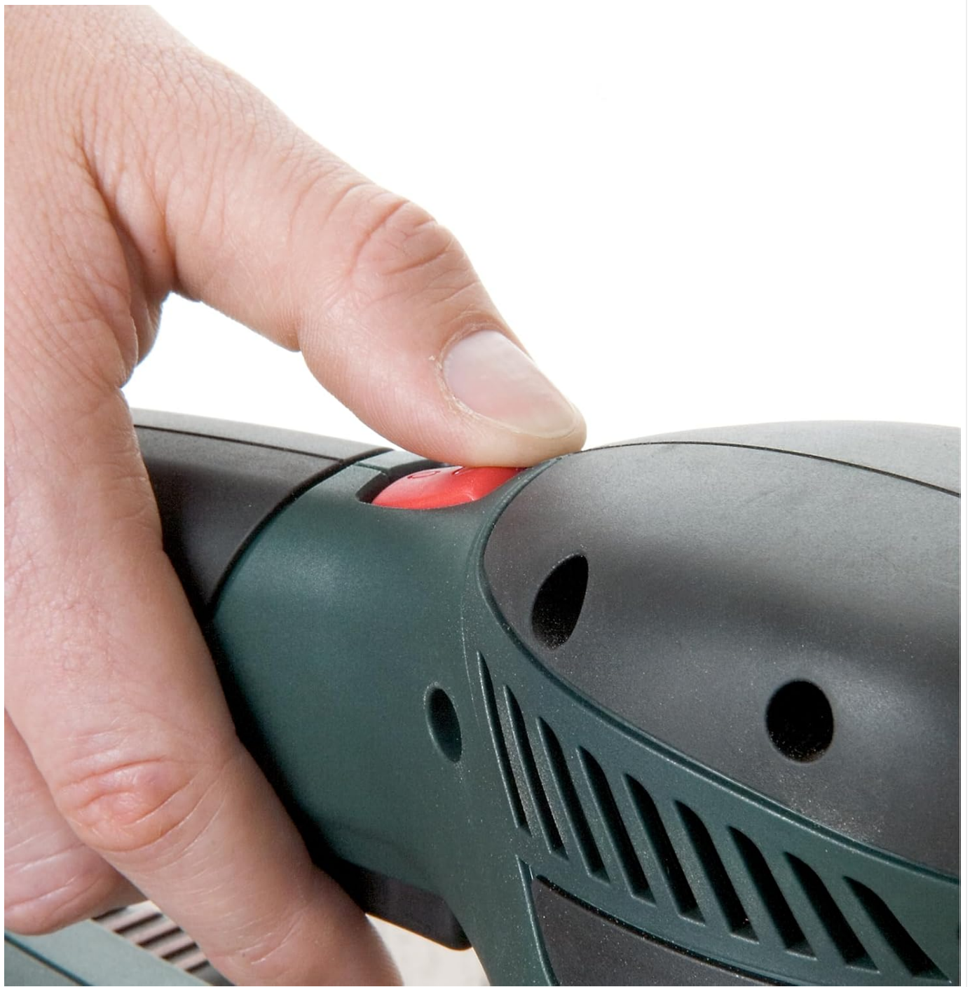
Figure 4.1: Detail of the power switch, indicating its location for easy access during operation.
